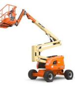
**General Precautions:** There should always be two people working together when operating mechanical lifts. Harness, hard hat, eye protection should be worn at all times. Check the bubble level to ensure ground is level. Check weather conditions before use. Inspect the equipment against the checklist daily, per job. Make sure the work area is demarcated and barricaded. The operations manual must be on the equipment at all times. Do not use less than 10 feet away from electrical power lines.
