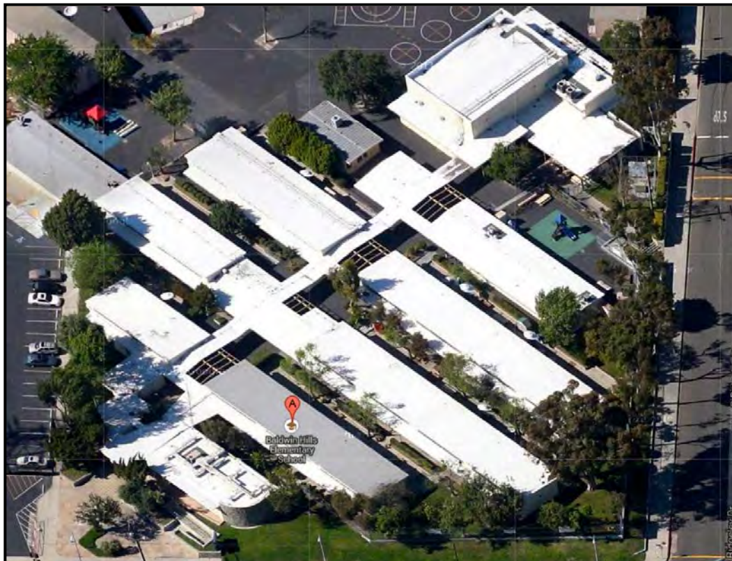
Figure 127. Neutra & Alexander, Baldwin Hills Elementary School. Aerial shows the condensed finger-plan design used to create the preferred one-story massing, set off by swaths of landscaping and patios, but with a more compact site plan. Source: Google Maps, 2013.
