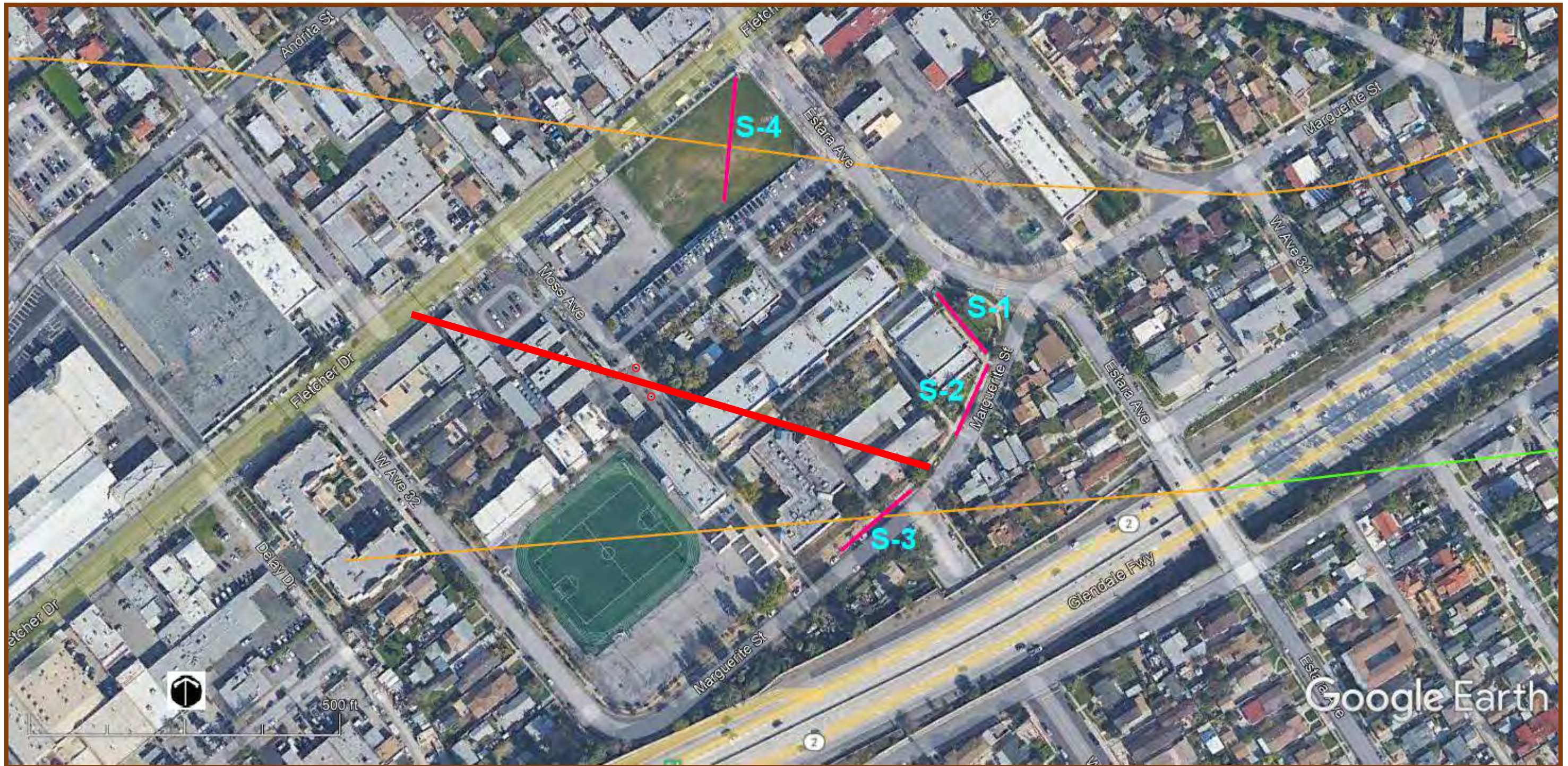
Base Map: Google™ Earth imagery (2021), Seismic Line S-1 through S-4 shown as red lines, approximate mapped fault locations shown as orange lines.
