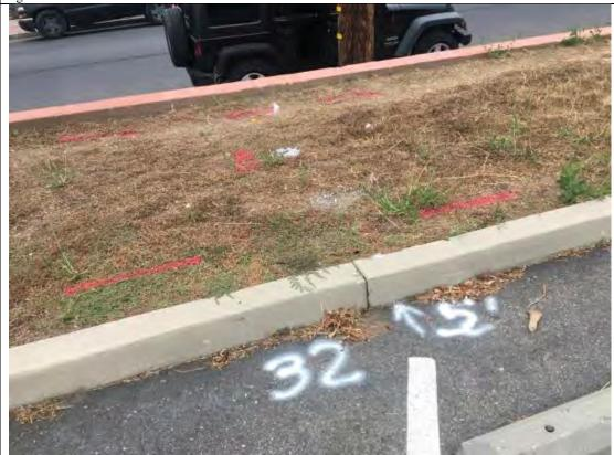
Photo 8: View WSW and down. Pin flag at SHS-32. Dieldrin concentration 22  $\mu$ g/kg in surface sample. Boring between street lighting electrical line trace (background) and unknown utility line trace (foreground).
