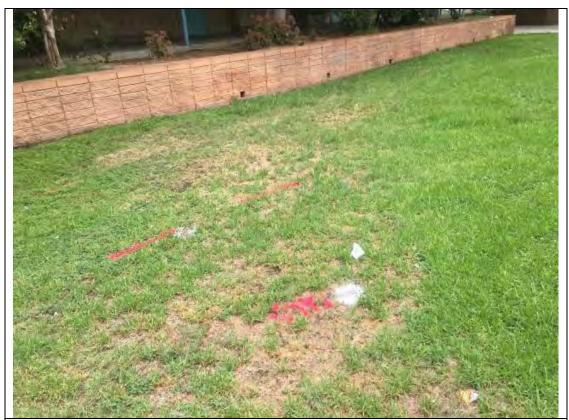
Photo 1: View SSE and down. Pin flag at SHS-03. Dieldrin concentration 32  $\mu$ g/kg in surface sample. Sewer line trace to rear.
