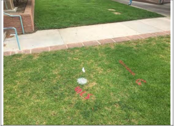
Photo 4: View SSE and down. Pin flag at SHS-27. Dieldrin concentration 83 µg/kg in surface sample. Gas line trace to right. Storm drain grate right background.
