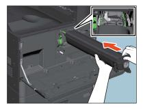
Carefully pull the cleaner out until it comes to a stop, and then carefully reinsert it straight into its original position. Repeat this step a couple of times.
