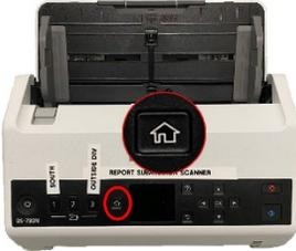
Press the Home Button to reset the scanner in preparation to send a new report
